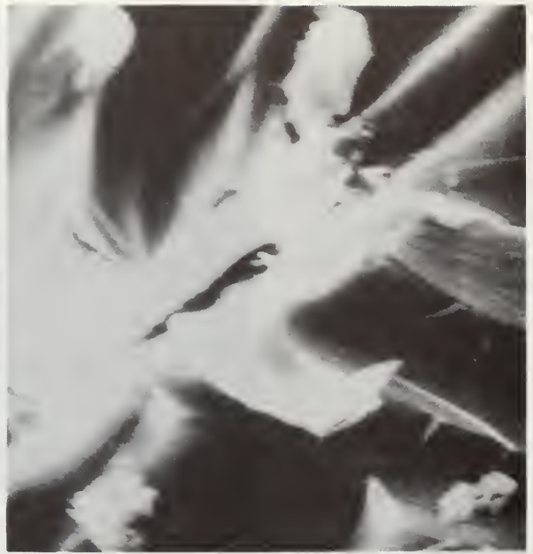
FIGURE 16. SCANNING ELECTRON MICROGRAPH OF THE FRACTURE SURFACE AT A FLAW OF A TENSILE SPECIMEN; EPON 828 + 10 pph CTBN 20-64 (SMALL PARTICLES) + 5 pph CURING AGENT D.
